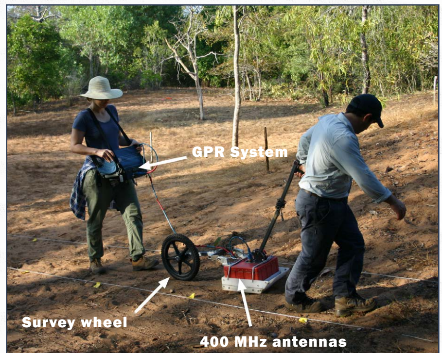
Key components of the GPR system
