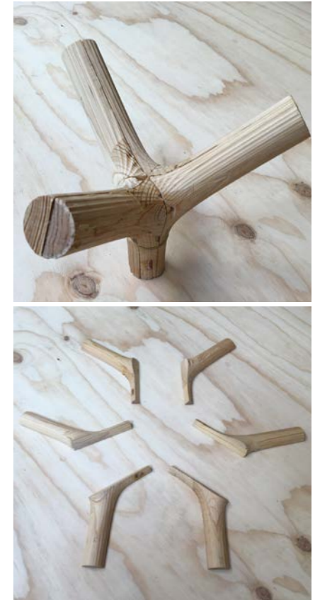
Above: A timber joint created using parametric modelling.
